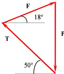
$$\frac{500}{\text{sen } 68^\circ} = \frac{F}{\text{sen } 40^\circ} = \frac{T}{\text{sen } 82^\circ} \quad F = 346,6 \text{ N}$$
