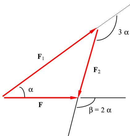
$$\alpha = 48,2^\circ \quad ; \quad \beta = 96,4^\circ \quad ; \quad F_1 = 1,7 F \quad ; \quad F_2 = 1,3 F$$
