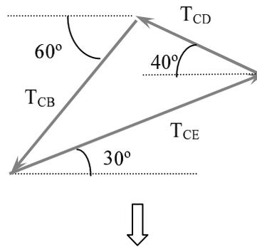
$$\frac{2450}{\text{sen } 60} = \frac{T_{BA}}{\text{sen } 30} = T_{BC} \quad ; \quad T_{BC} = T_{CB} \quad ; \quad \frac{T_{CD}}{\text{sen } 30} = \frac{T_{CB}}{\text{sen } 70} = \frac{T_{CE}}{\text{sen } 80}$$
