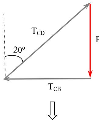
$$\frac{500}{\text{sen } 10} = \frac{T_{BC}}{\text{sen } 80^\circ} = T_{BA} \quad ; \quad T_{BC} = T_{CB} \quad ; \quad \frac{P}{\text{sen } 70} = \frac{T_{CB}}{\text{sen } 20^\circ} = T_{CD}$$
