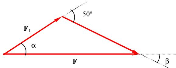
$$F_1 = 6,18 \text{ kN} \quad ; \quad F_2 = 15,45 \text{ kN} \quad ; \quad \alpha = 36,2^\circ \quad ; \quad \beta = 13,8^\circ$$
